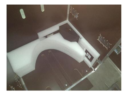
13. Place the mold elements, fixating plates and other removed constituent parts of the protective case in the case. Place the lid on top of the case and fixate it. Keep the protective case to be used for robot's handling and transportation in the future.
