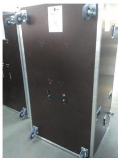
3. The case should be handled strictly vertically (as marked on the label), or rolled on its wheels when handled horizontally;
