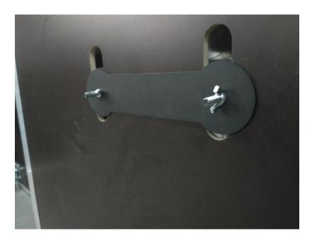
6. Remove the carrier (fixating) plate;
