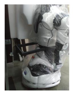
When accepting the delivered robot remember to make sure that the protective case has been handled properly (vertically, as labeled, or on wheels when handled horizontally), and check the case for any possible damage in transit. **Unpack the case with an assistant!**
